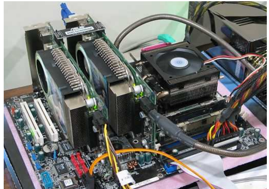
A 2 GPU system using NVIDIA SLI.
