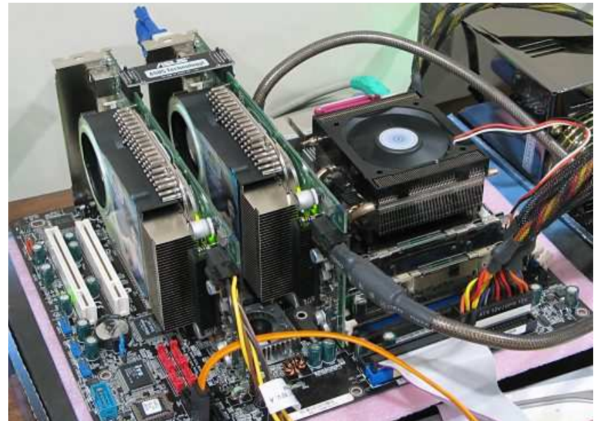
A 2 GPU system using NVIDIA SLI.
